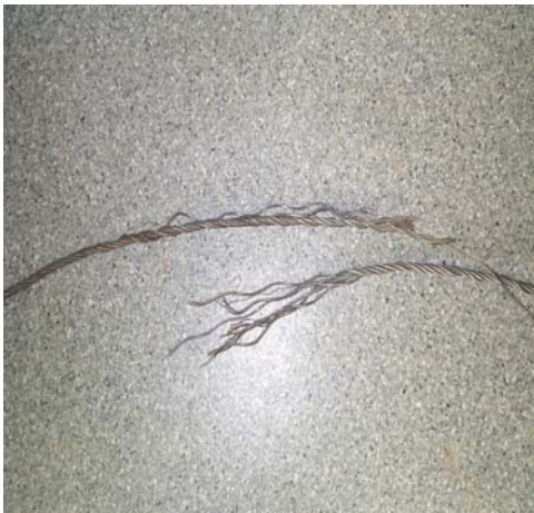
Figure 3. 8mm diameter, 6 strand wire cable showing tensional failure.
