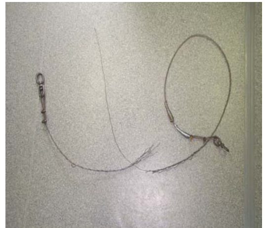
Figure 4. Lifting 'rope' showing failure and twin swivel set-up.
