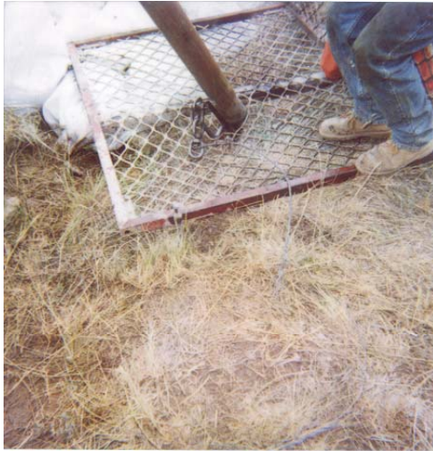
Figure 1. Metal mesh guard on which off-sider struck knee. Lifting hook with handle still in rod end, failed wire rope and swivel attached.
