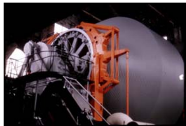
Cone Winder on a deep incline shaft near Marquette, Michigan, 1968
