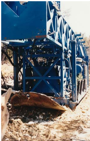
Because the track was so soft and the rig so heavy a "shoe" used for skidding logs was borrowed and used to stop the skid frame from digging in.
